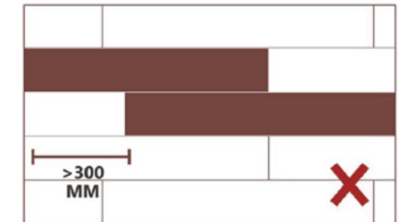
The longest side should be staggered no more than 300mm when laid in running bond.
